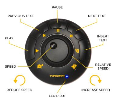
**NOTE:** In teleprompter systems using the XPRO version of our software, an adapted version of the Shuttle will be provided, replacing the *Play* and *Insert Text* buttons with *Reverse Direction* ♣ and *Fast Forward* ▶ respectively.
