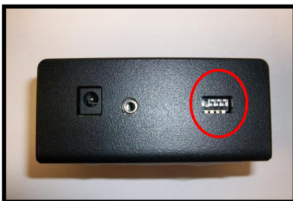
Figure 5. Switches to configure the displayed number
